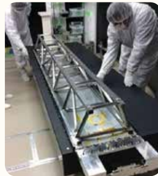
Constructed iTOP module augmented by external "strong back" to stiffen it until installation. Sixteen such modules will form a cylinder within the Belle II detector. The last module is slated for installation in spring 2016.
